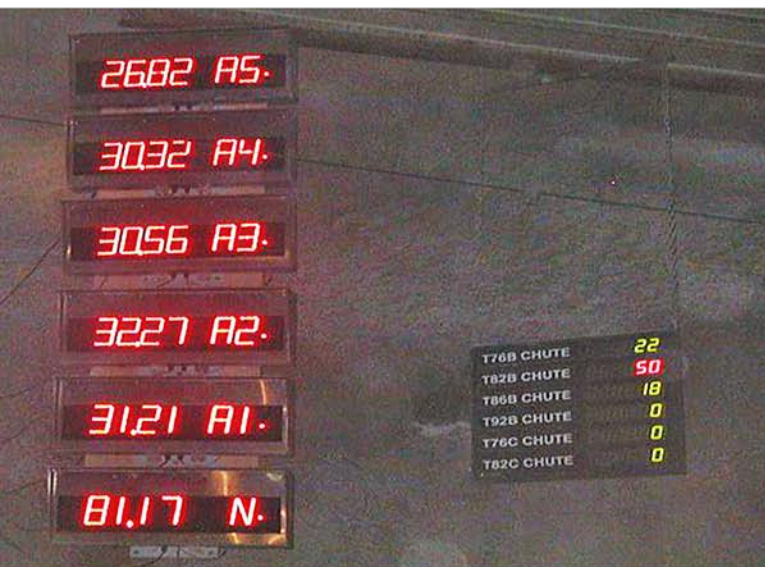
Axle and net weight displays and chute status displays at crusher site.
