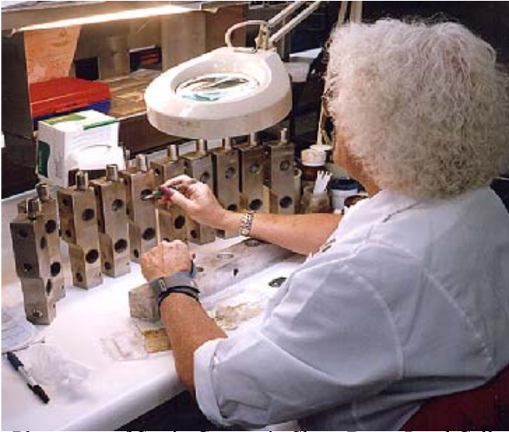
Placement of Strain Gauges in Shear Beam Load Cell
