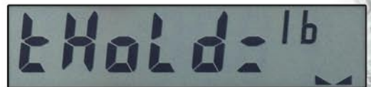
Checkweigher which does not allow PWC outputs until a specified number of pieces are applied to the scale.
