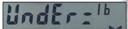
Checkweigh operation with hopper fill and dump with dump timer, settle timer, and zero timer.
