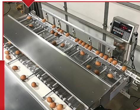
**3** Programmed into the 210 indicator are six preset egg weights determined by the operator.
