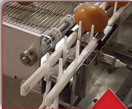
**1** Eggs are optically scanned for placement and weighed, which is read and stored in the 210 indicator.
